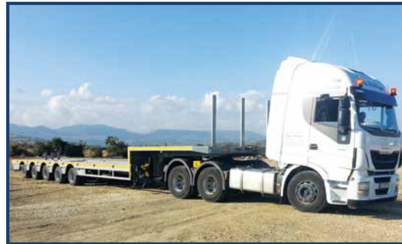
Trafo Dorsesi / Transformer Trailer
